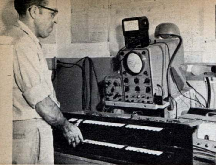
Electronics engineer Percy Stewart must check each tone wave against a standard wave form on an oscilloscope before final assembly of organ.
